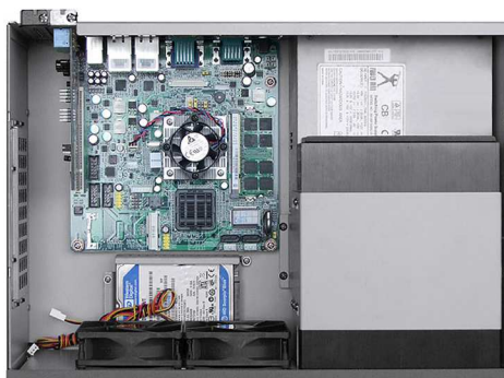
PS2 power supply installed mode
