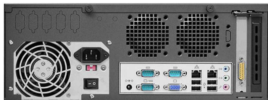
PS2 power supply installed mode
