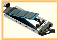
Push the front angle hook and press downward the M.2 SSD
