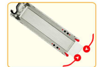
Press the plastic holders and release the heat sink
