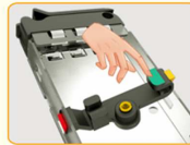
Insert the left bump into the left square hole at 45° angle, press side angle hook, the right bump is fixed
