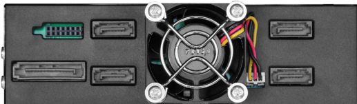
Four SATA 7pin data transfer ports
